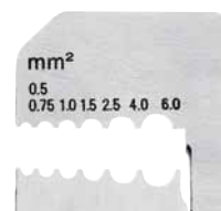
12 21 180: wire cross-sections in mm²
