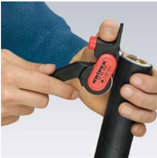
Setting the tool for longitudinal cut
