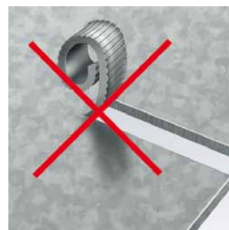
Notching without chip breaking
