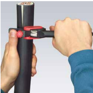
Turning the tool for circumferential cut
